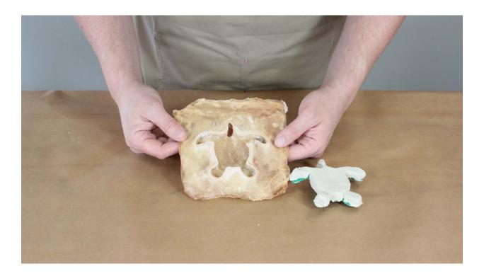
20. A freeze and fuse casting made in the latex mold.
